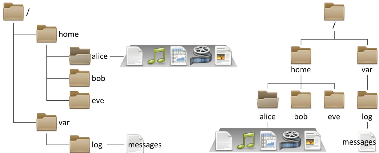
Figure 2.2: The common file browser view (left) is equivalent to the top-down view (right)
