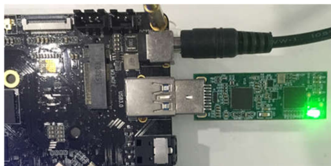
Figure 7. USB Compute Stick plugged into USB3.0/SS port of ARM platform
