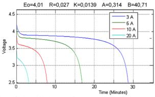
Figure 4 Discharge of the battery at different currents (nominal discharge current is 0.65 A)
