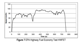
The calculation of the necessary energy is carried out it is energy that mechanically burdens the EV drive, based on the driving mode and the basic parameters of the EV. This energy is transferred through electric drive and is considered as the electrical load of the battery (*discharge* acceleration and driving, *charge* - recovery of braking energy).
