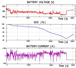
Figure 15 Change parameters battery pack for UDDS + HWFET drive cycles
