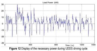
The diagram in Fig. 12 provides an overview of changes in power that EV drive must provide for UDDC drive cycle.
