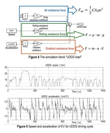
The value of C (drag coefficient: 0.0425) and A (an area of the front side of the vehicle) are taken from Mitsubishi i-MiEV that is based vehicle model in this paper.
