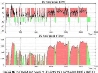
Figure 16 The speed and power of DC motor for a combined UDDC + HWFET drive cycles.
